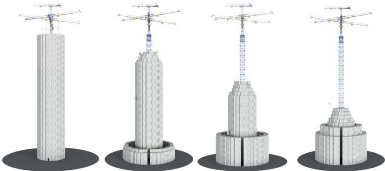
Figure 44: Energy vault system of piling blocks
