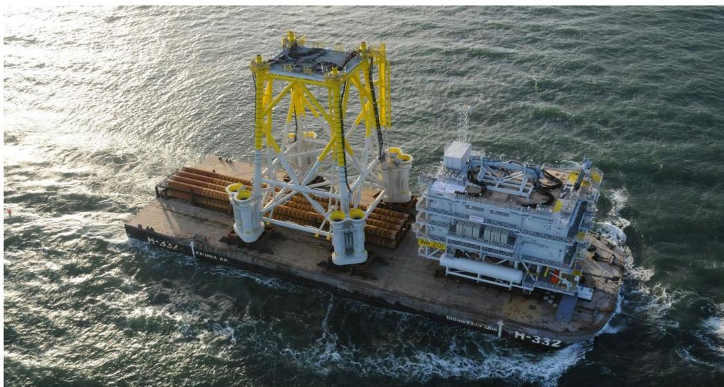
Figure 5-6: Offshore substation top side and sub-structure [10]
