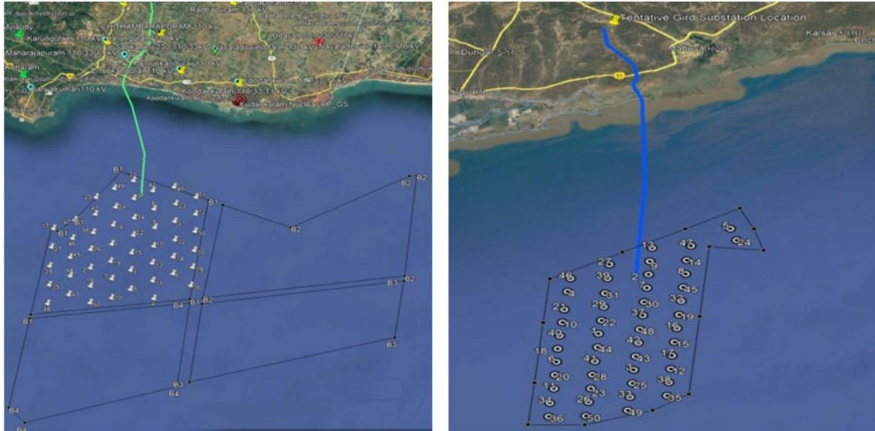
**Figure 5-10: Layout of WTGs of 1GW OWF in Tamil Nadu (left) and Gujarat (Right)**
