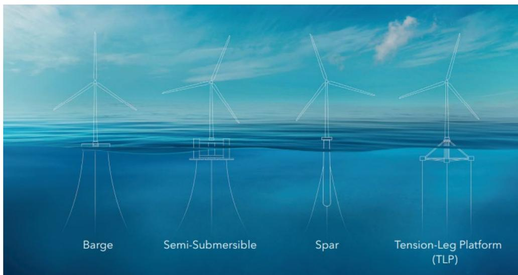
Figure 4-10 Floating Foundation Types
