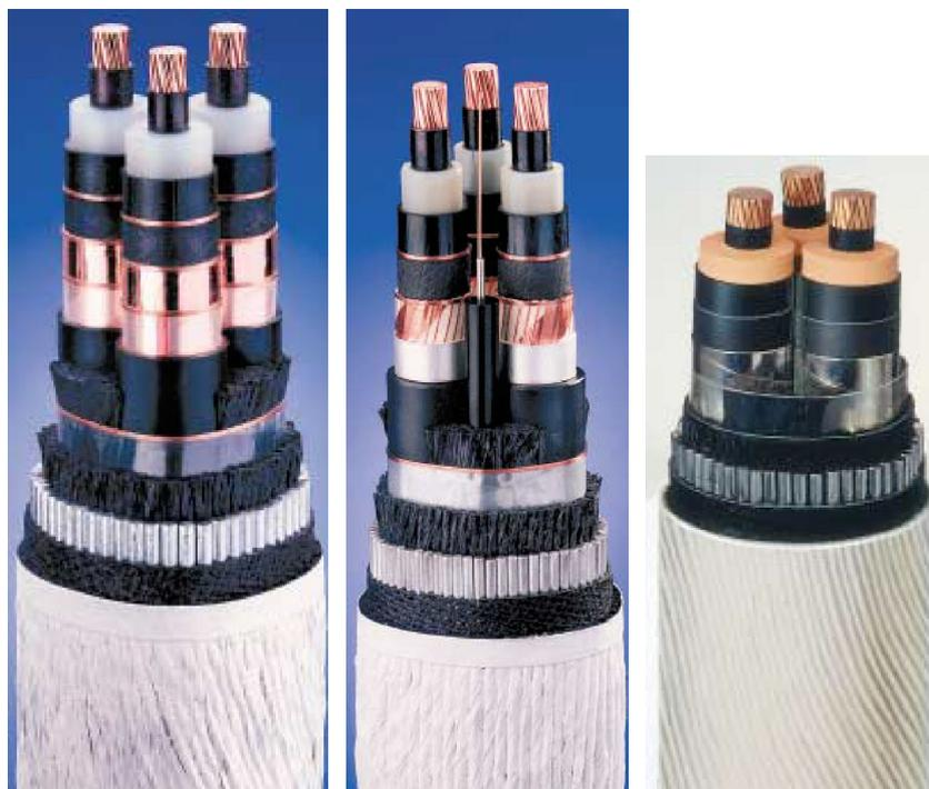
Figure 5-5: (left) Medium-voltage submarine cable, XLPE insulated; (middle) Medium-voltage submarine cable, including fibre optic cable; (right) Medium-voltage submarine cable, EPR insulated [9]
