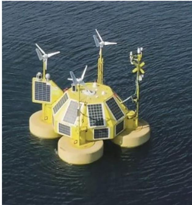
**Figure 5-12 Floating Lidar system (FLS) [13]**
