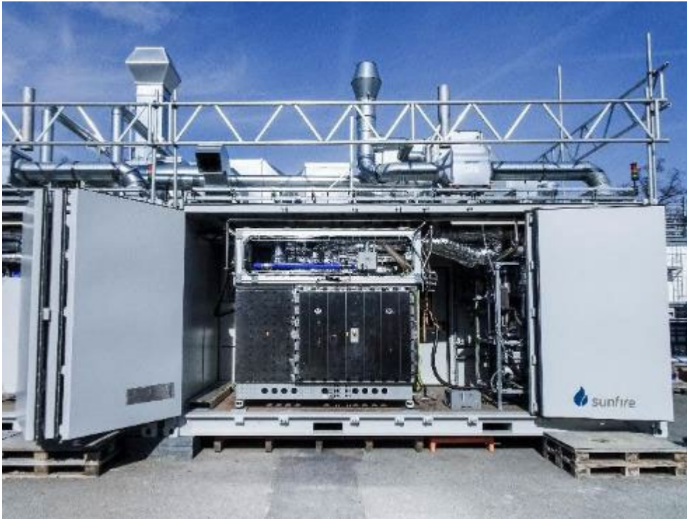
Figure 189: Sunfire's SOEC Module "Generation 2" (225 kW) (Source: Sunfire GmbH)
