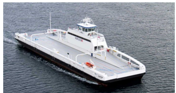
Figure 155 - World's first electric ferry, Ampere, constructed for Norled by the Norwegian Shipyard Fjellstrand 4
