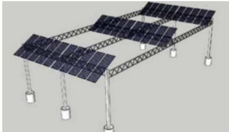
Figure 3: Overhead east west APV configuration
