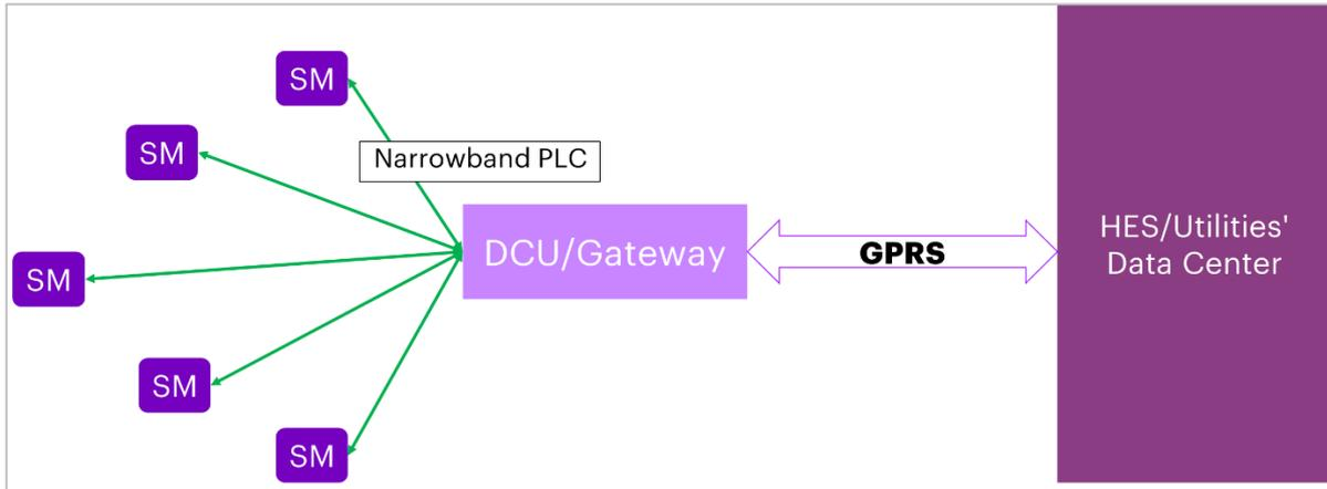
**Figure 19: Architecture deployed by CenterPoint Energy (Houston, USA)**
