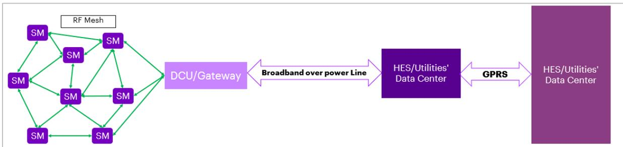
**Figure 20: Typical AMI architecture with RF mesh as last mile**
