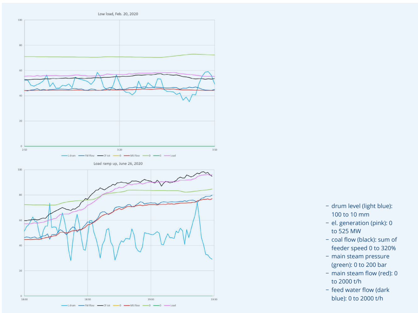
Figure 7: Main plant parameters during low load operation (above) and ramp up (below)
