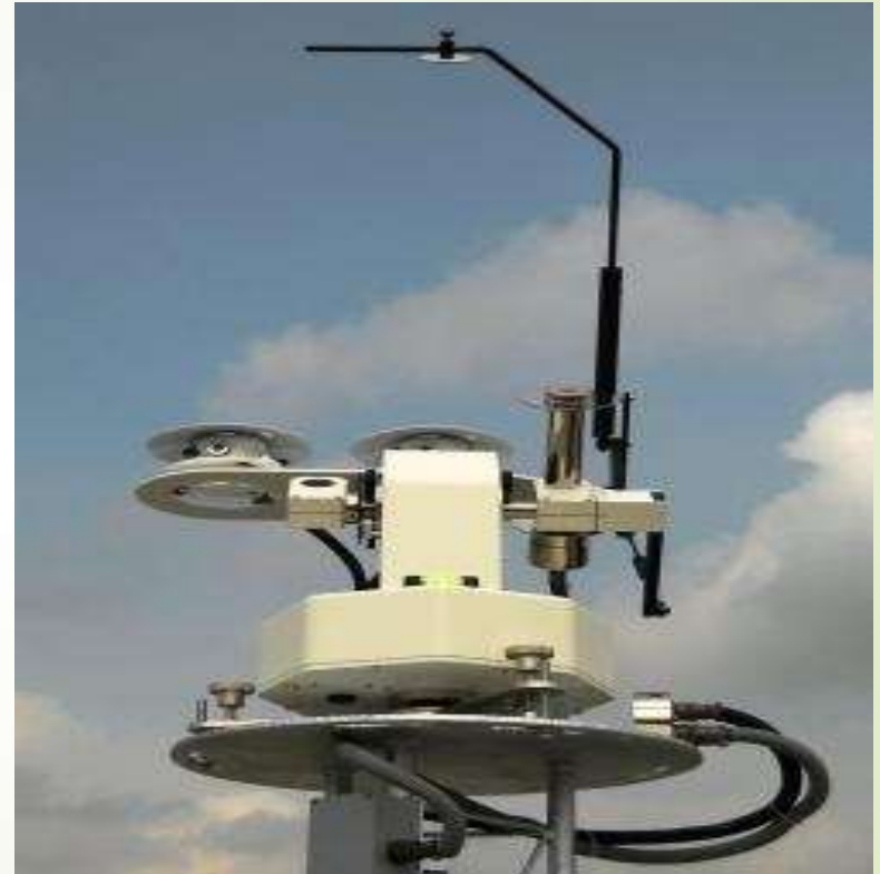
Sun tracker with solar radiation measurement equipment
